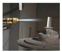
The automotive and aerospace industries some mechanical parts are highly loaded with temperatures, corrosion and erosion. To protect them against these heavy influences, plasma spraying is the solution.
